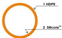
Wall thickness and material classify the duct as a Direct Burial (DB). Installation methods and conditions are described in the Installation manual.
